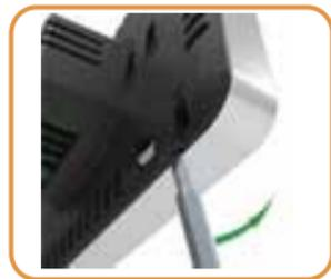
Separate the panel from the back section: insert the screwdriver into two holes under the thermostat and pry it like the picture.
