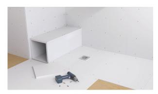
In addition to 15mm wall boards, Aqua4ma panels are available in 7mm panels for flooring and solid walls and 25mm for more structural requirements such as seats and shelves. These can be screwed into place and permanently bonded with Aqua4ma solvent weld paste for guaranteed watertight joints.
