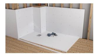
Aqua4ma Evolution shower decks are easy to trim, either to fit the available size, or to shape around ducting etc. Aqua4ma 15mm tongue and groove wall panels can be screwed directly to battens in place of plasterboard and, as the material self seals around screws, no washers or additional sealing is neccessary. Aqua4ma panels also provide stable fixing for accessories.
