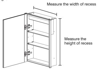
1.2 - Mark out the recess on the wall. Special attention must be taken to ensure there is nothing within the desired recessed space.
