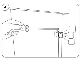
If the delivered configuration isn't suitable, remove door from unit using a suitable tool.
